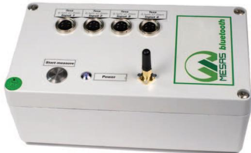
**Wireless transmission** of measuring data from the interface box to the measuring computer **by Bluetooth® technology**.
