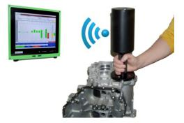
Application Example: Diameter and depth on a transmission housing with 12 transducers
